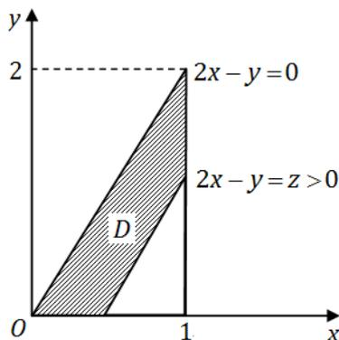
$$\begin{aligned} F_Z(z) &= P\{2X - Y \leq z\} = \iint_{2x-y \leq z} f(x, y) dx dy \\ &= 1 - \iint_{2x-y > z} f(x, y) dx dy = 1 - \int_{\frac{z}{2}}^1 dx \int_0^{2x-z} dy = z - \frac{1}{4}z^2. \end{aligned}$$
